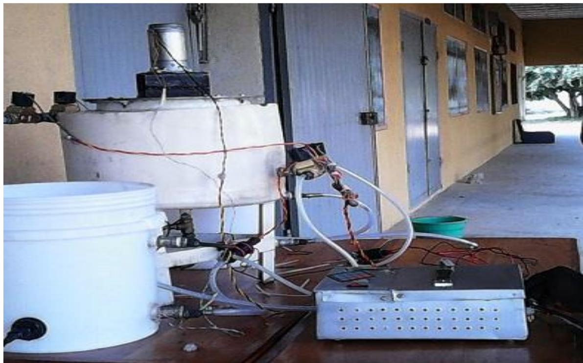
Figure 1. Biodiesel batch reactor constructed for this work.
