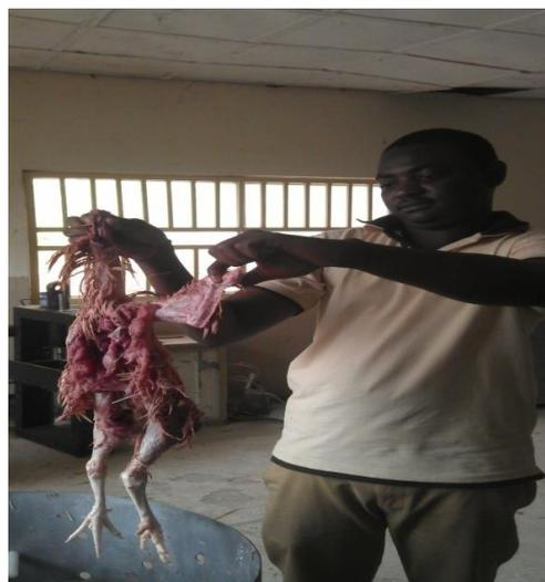
**Plate II:** One of the chickens damaged by the existing machine
