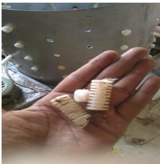
**Plate I:** Some broken fingers of the existing machine
