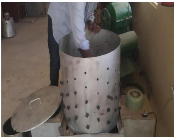
Plate III: The modified de-feathering machine
