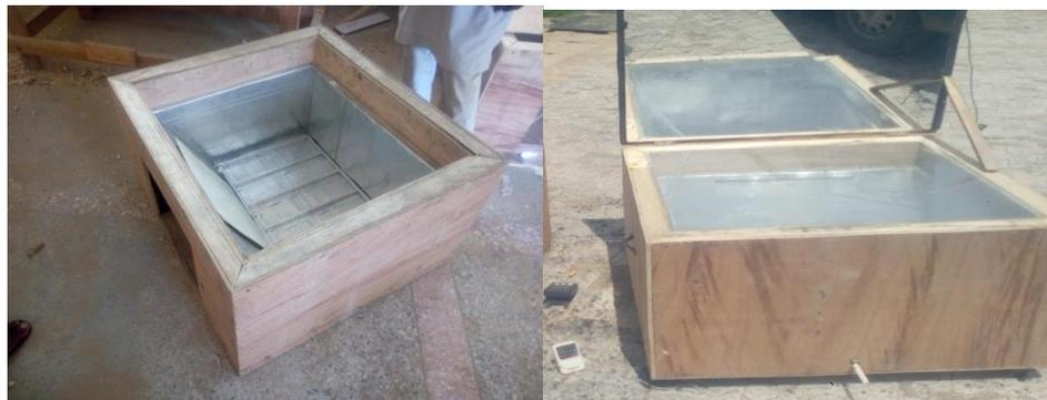
Plate 1. Box unit with PCM tank before (a) and after glazing(b)
