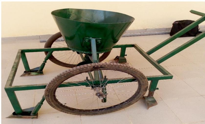
Plate 1. Pictorial View of the Constructed Two Row Single Metering Plate Maize Planter
