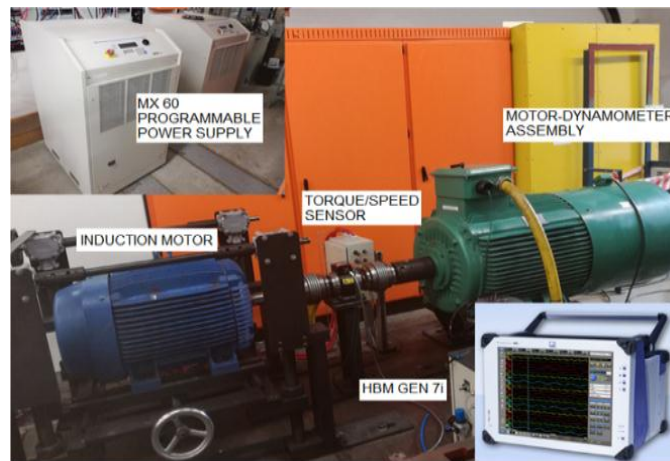
Figure 4. The complete 110kW laboratory test bench showing all the system components
