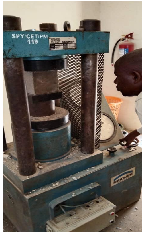
Plate 4. Compressive Test using Compressive Test Machine Seidner SWP200EMI Model
