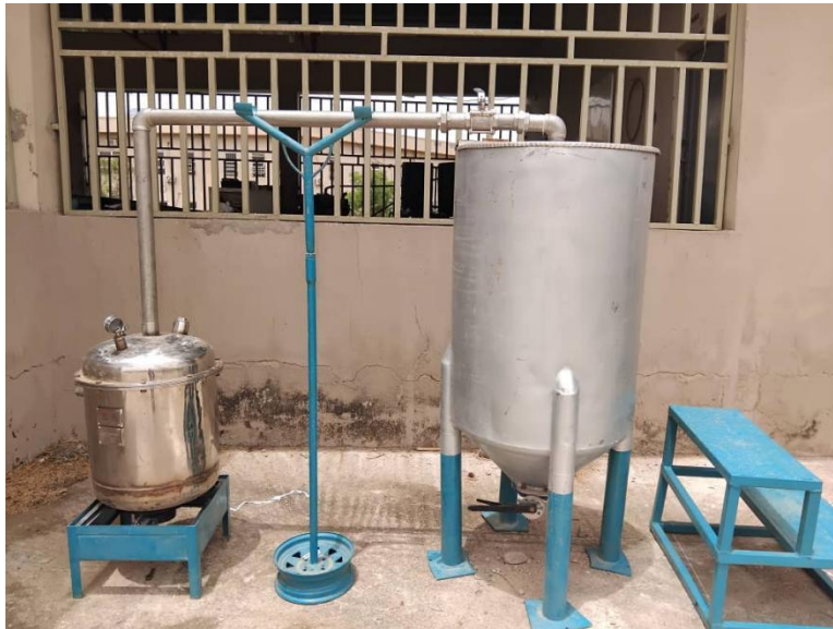
Plate 1. Pictorial View of the Developed Paddy Parboiler
