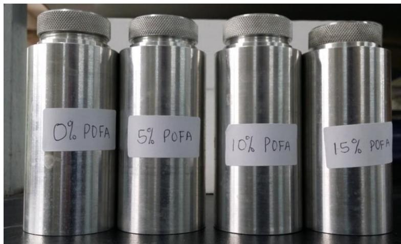
Plate1: Modified moulds used in the centrifuge
