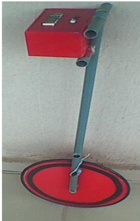
Figure 6. The constructed Digital Surveyors wheel
