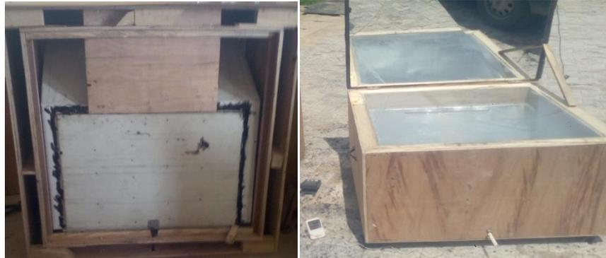
Figure 4: Box unit with PCM tank where heat transfer takes place in position before and after glazing
