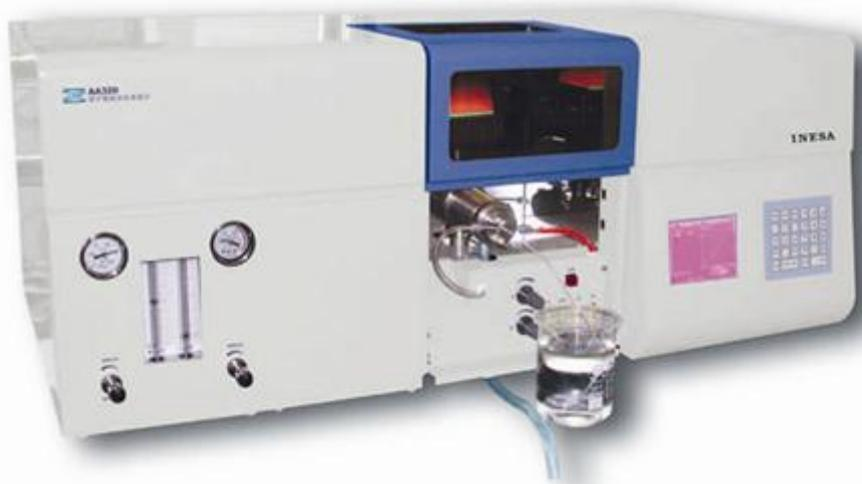
Plate 2. GA3202 HGA Graphite Furnace System
