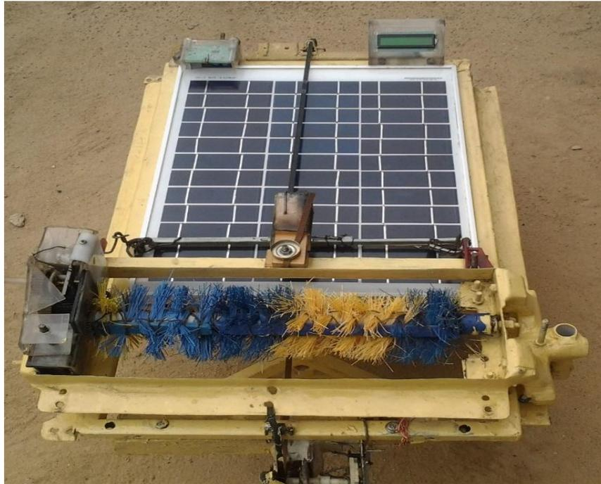
Figure 6. Constructed solar cleaning system
