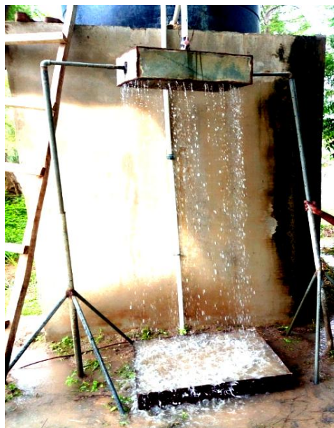
Plate 1. The Modified Rainfall Simulator
