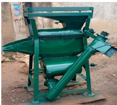
Plate I. Full assembly of the developed motorized maize thresher
