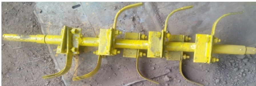
Figure 6. Shaft and Shredding Blades Assembly of the Developed Shredder
