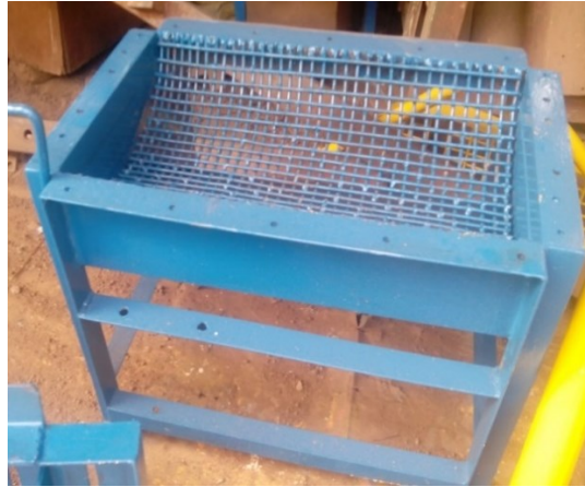
Figure 5. Frame and Screen Assembly of the Developed Shredder
