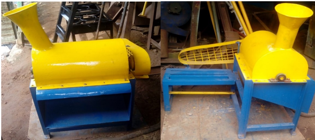
Figure 4. Front and Rear Sides of the Developed Shredder
