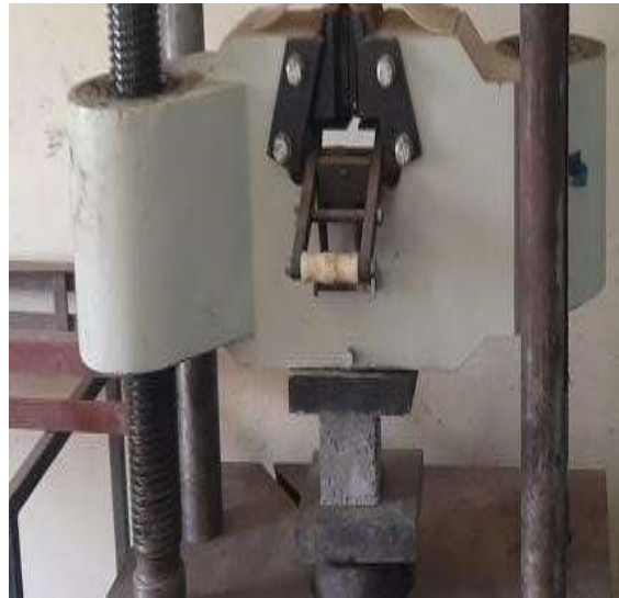
Plate 6. Compressive Test using Zhejiang Tugong Universal Testing Machine
