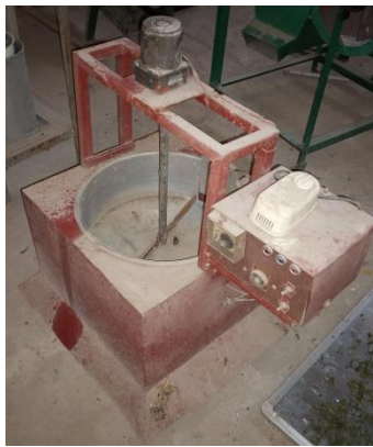
Plate 1. Constructed Vertical Paddle Rotary Gari Frying Machine
