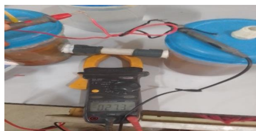
Figure 2b. Open circuit current reading
