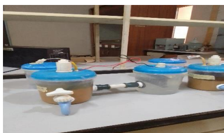
Figure 2a. Set up of H-shaped microbial fuel cell
