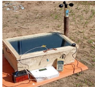
Plate 3. IoT monitoring interface on solar box cooker experiment
