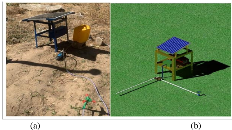
Figure 5. Fabricated Model (a) and Computer aided Design (b) (CAD) Model of Smart Solar Irrigation System showing Monocrystalline Panel in position
